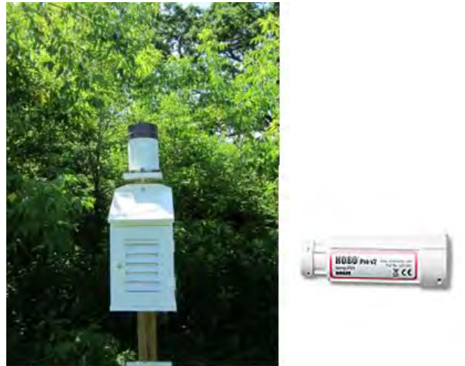
Fig. 8. A weather station with instrumentation for continuous monitoring of air temperature, relative humidity, dew point (right), and rainfall.
