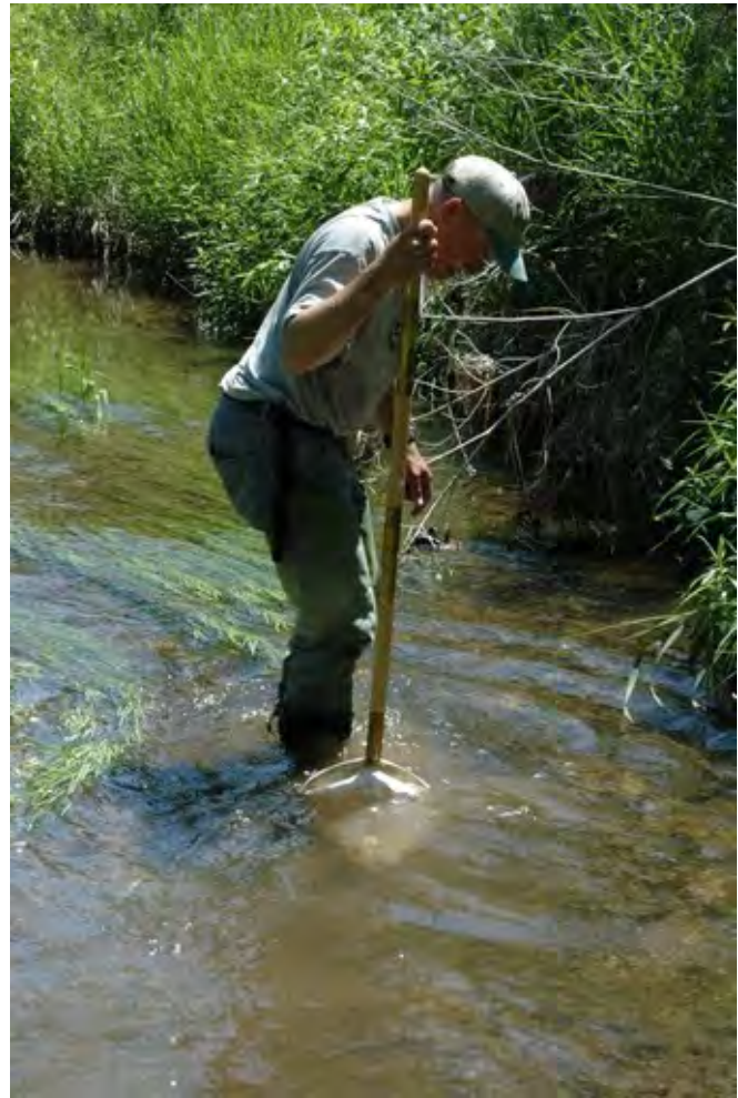
Fig. 11. Using a kick-sampling protocol to collect a macroinvertebrate sample at a stream restoration monitoring site.
