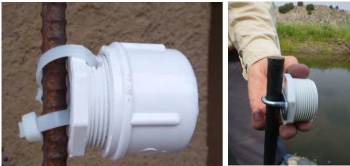
FIGURE 6. PVC HOUSING FIXED TO REBAR USING A NYLON STRAP (LEFT), OR ALTERNATIVELY FIXED TO A COLD ROLLED STEEL BAR USING A U-BOLT (RIGHT).
