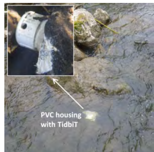
FIGURE 7. PVC HOUSING EPOXIED TO A ROCK.
