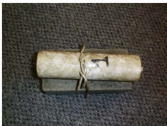
In PVC tube attached to brick
