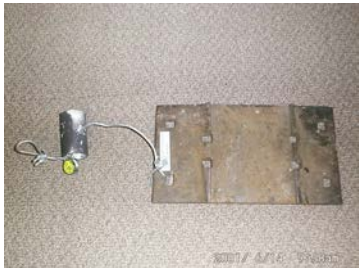
Connected to railroad tie plate and protected by PVC tube
