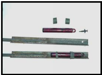
Connected to angle iron welded to re-bar and pounded into stream bottom
