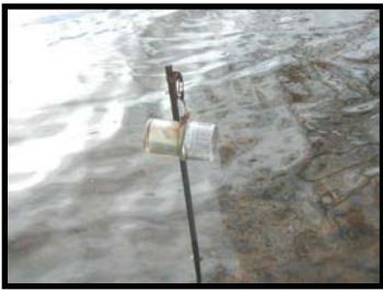
In capsule attached to fence post or re-bar and pounded into stream bottom
