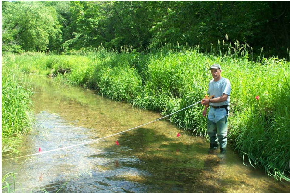
Measuring stream width and marking quarter-point locations within the 1-meter wide transect at Lower Pine Creek_T6L
