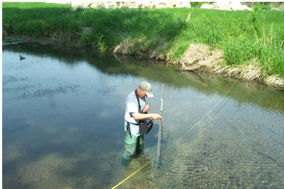
Measuring water velocity at a quarter-point location within the 1-meter wide transect at Lower Pine Creek_T1L
